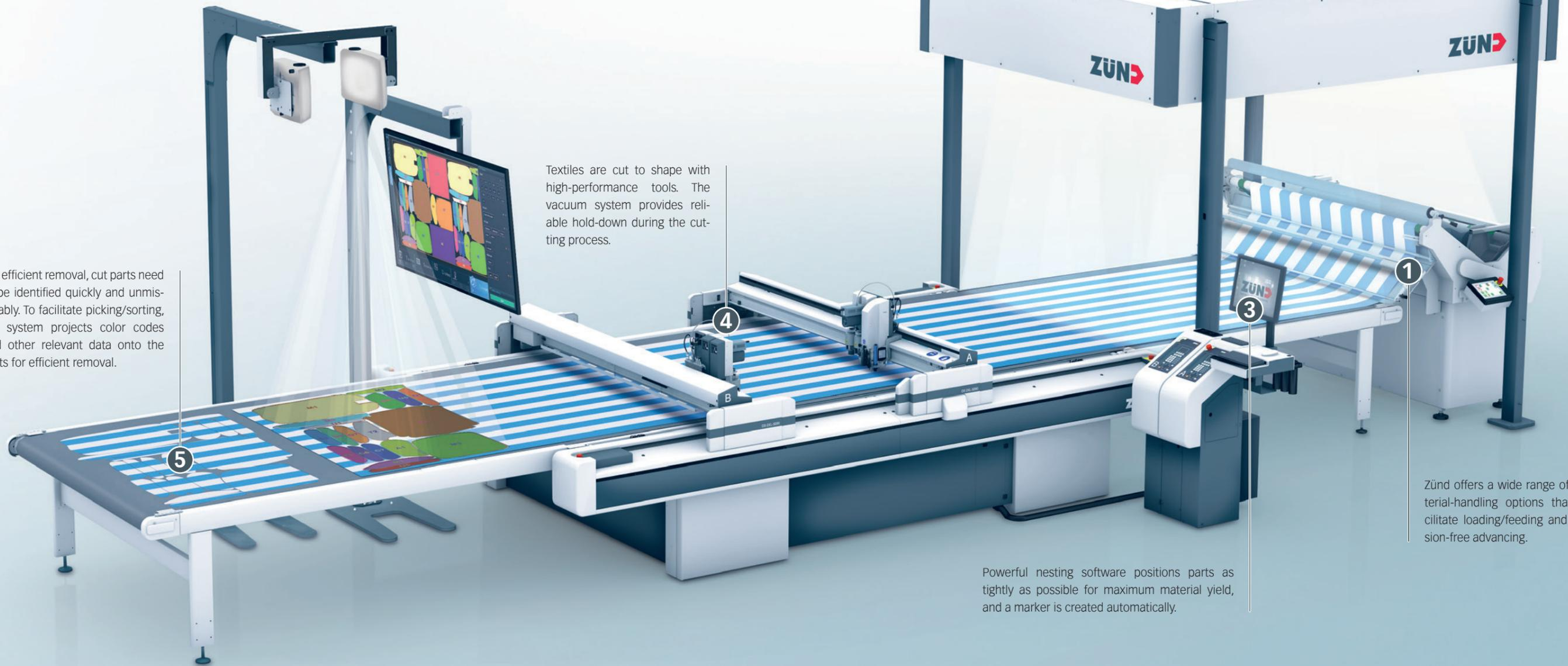
For efficient removal, cut parts need to be identified quickly and unmistakably. To facilitate picking/sorting, the system projects color codes and other relevant data onto the parts for efficient removal.
